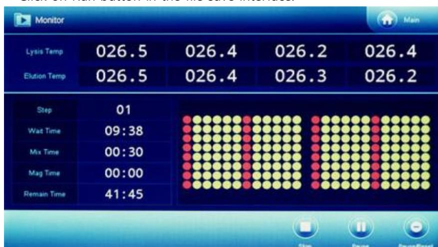
The lysis and elution temperatures are displayed on top of the running interface. The lower left side of the interface shows the steps undergoing, including waiting time, mixing time, binding time, and remaining time.
